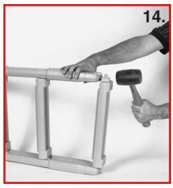
Attach the two remaining standard treads to the extension boots (or directly to the ends of the ladder legs if installing on a 48" tall pool).
