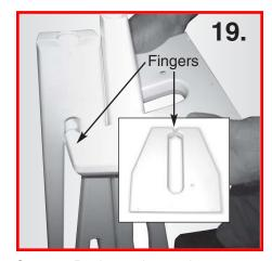
Separate Barrier sections at the top slightly and position Upper Brace over Small Barrier Section. Next, spread the "fingers" on the Upper Brace and slide into position on the Large Barrier Section.
