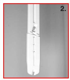
Slip the four extension boots over the ends of the assembled ladders legs. They will need to be all the way on for most 52" tall pools and backed off one hole for 54" pools. Depending upon ground levels outside the pool, and sand levels under the liner inside the pool, a final adjustment may need to be made after the ladder is put into place.
