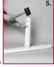
Push the end of one of the standard treads into the uppermost keyhole slot. Make sure that the tread and the ladder leg are positioned as shown in the photograph above. It may be necessary to tap the tread into the slot with a mallet. Repeat for three additional treads.
