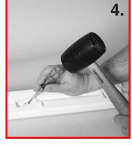
Remove the keyhole slot inserts from two of the ladder legs.
