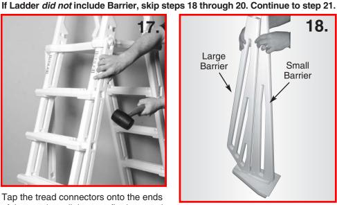
Snap Small and Large Barrier Sections into slots on Lower Base as shown.
