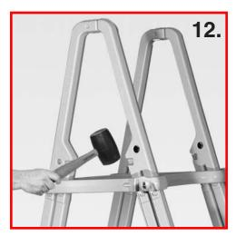
Tap the platform down until it is fully seated on the "lugs" of the legs as shown.
