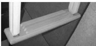
**6. Attach the upper tread included with this kit to the extension boots using two #10 x 1-1/2" screws left over from the assembly of the ladder.**
