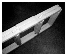
4. Drill two 5/16" holes all the way through each extension boot and fasten with the ½-20 x 2" bolts and acorn nuts. Drill one of the holes near the top of the sleeve section of the boot and the second hole near the bottom of the sleeve section.
