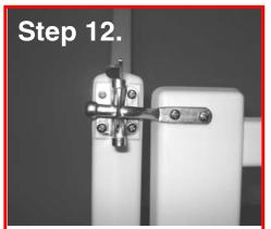
With the gate closed align the bar/plate by locking round end into the latch and holding flat end with two holes level on the gate. Fasten using two (2) #10 x 1-1/4" self tapping screws.
