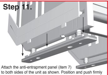
to both sides of the unit as shown. Position and push firmly down into base until it locks securely into place. Note: Anti-Entrapment panels are not needed if the unit is left at 48".
