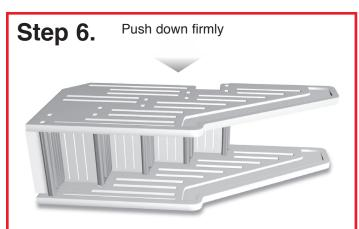
Push the second side panel firmly down on the step protrusions. It may be necessary to tap the side panel using a hammer and block of wood until seated correctly.
