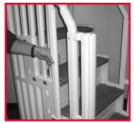
Align one of the triple pickets into the notches of the handrail at the top of the unit. Fasten the pickets in place at the top of the pickets using the #10 x 3/4" screws. Continue placing and fastening the double pickets and then the single picket. Repeat for the opposite handrail. Cover the ends of the screws with the protective caps.
