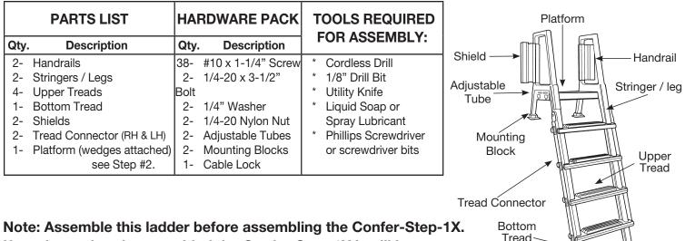
Note: Assemble this ladder before assembling the Confer-Step-1X. If you have already assembled the Confer-Step-1X it will be necessary to remove the handrails (see step #10).
