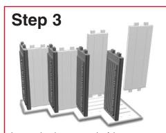
Insert a riser between each of the steps so that the ends of the risers align in the riser recesses on the same panel.
